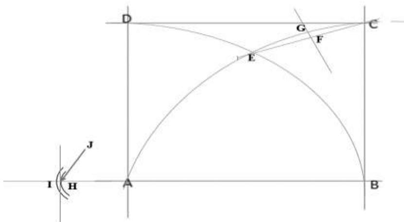
Figure 11: How to construct a line segment of length  $1.2599 \cong \sqrt[3]{2}$
