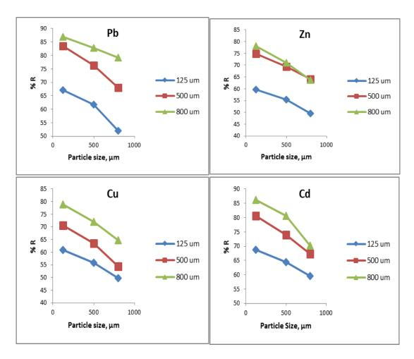
Figure 2. Effect of particle size on biosorption of Pb, Zn, Cu, and Cd onto palm leaves activated carbon The influence of initial concentration on metal ion biosorption (Biosorption Isotherms)
