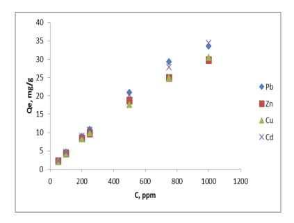
Figure 3. Effect of initial concentration on metal ion biosorption onto palm leaves activated carbon
