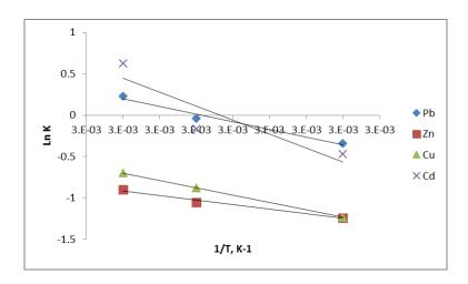
Figure 7. Plots of InK against 1/T for metal ions biosorption onto palm leaves activated carbon
