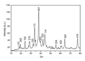
Fig2: X-ray Diffraction of Silver nanoparticle
