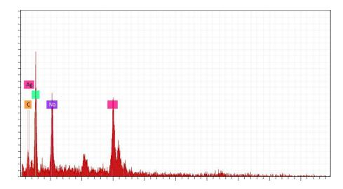
Fig 5: EDX spectra of silver nanoparticles
