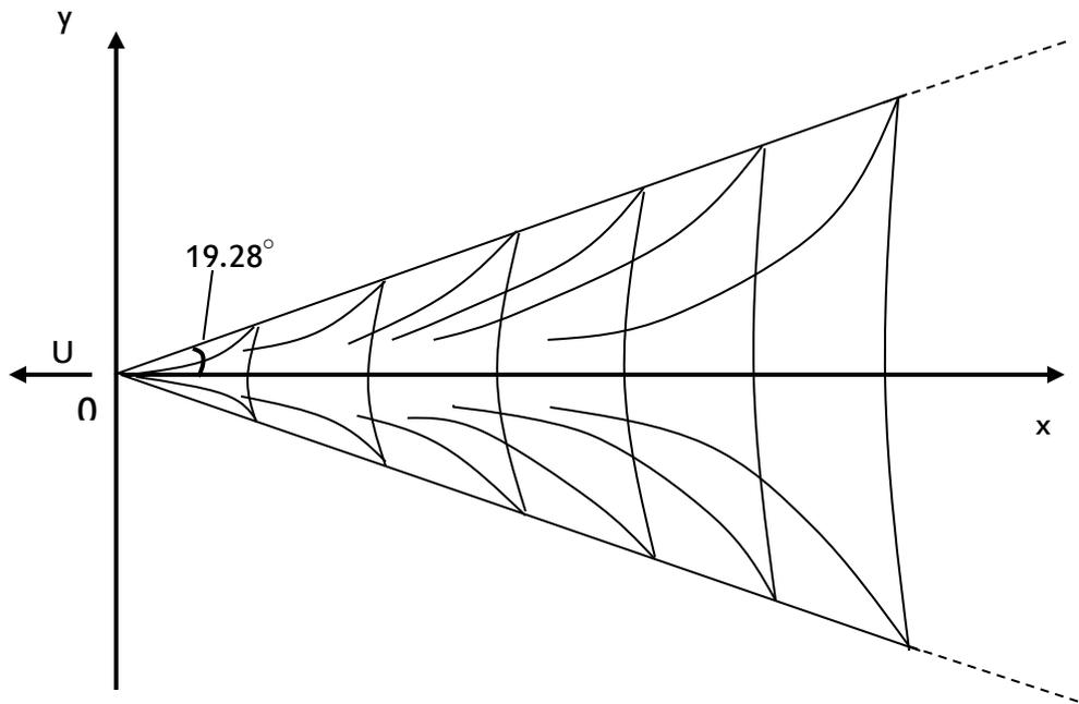
Fig. 4 Gravity wave patterns generated by a moving duck or ship with constant velocity  $U$ .
