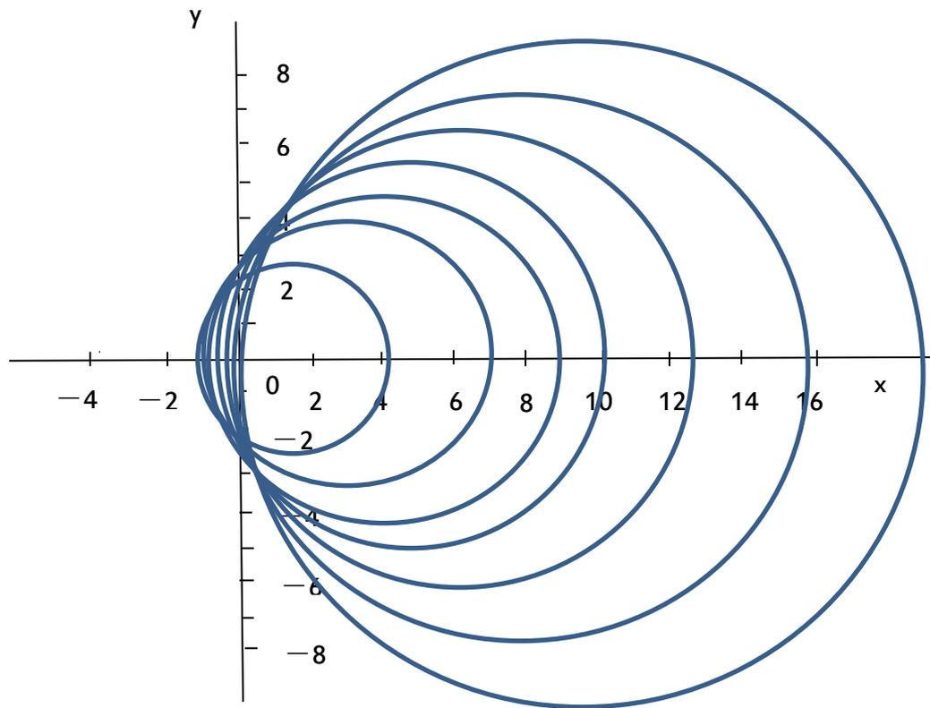
Fig. 1 An envelope of capillary waves generated by a moving point source, or stationary point source in the water stream with a constant speed.
