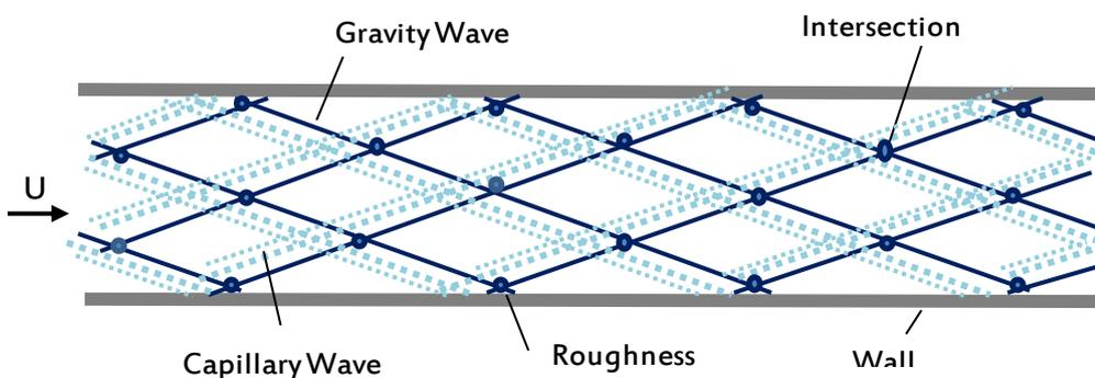
**Fig. 3 Sketch of interactions among gravity waves and capillary waves on the water surface in a channel.**
