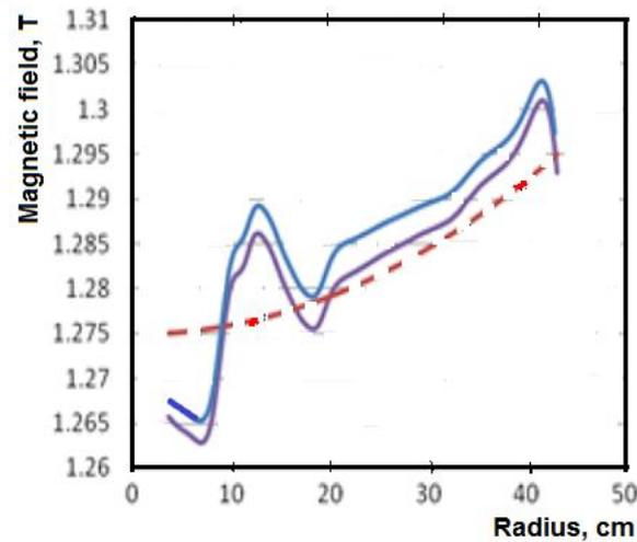
Fig. 6. The measured magnetic field (using two hall probes, solid lines) and isochronous magnetic field (dashed line).
