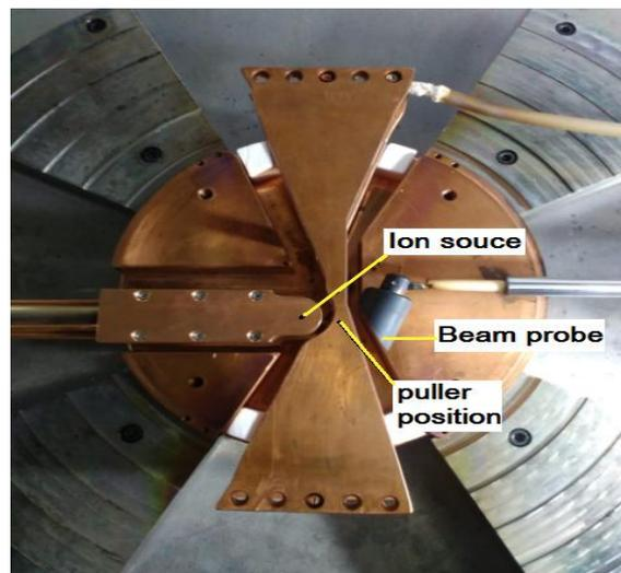
Fig. 4. Photograph of ion source testing in the central region of the cyclotron.
