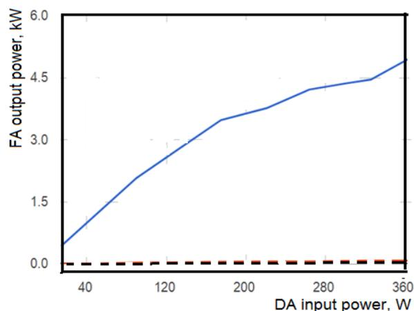
Fig. 8. The forward power (solid line) and reflected power (dashed line) of rf generator.
