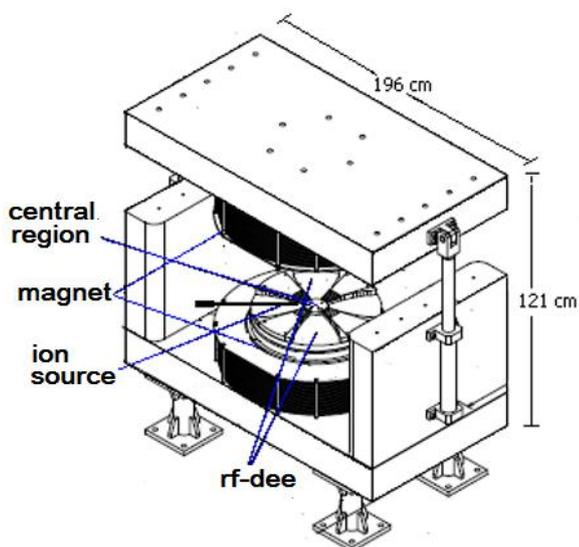
Fig. 1. The cyclotron architecture of DECY-13 Cyclotron
