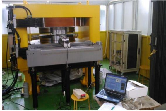
Fig. 3. The device for mapping magnetic field in the cyclotron
