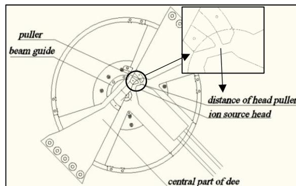
Fig. 2. The scheme of the central region of Dcy-13 cyclotron [12].
