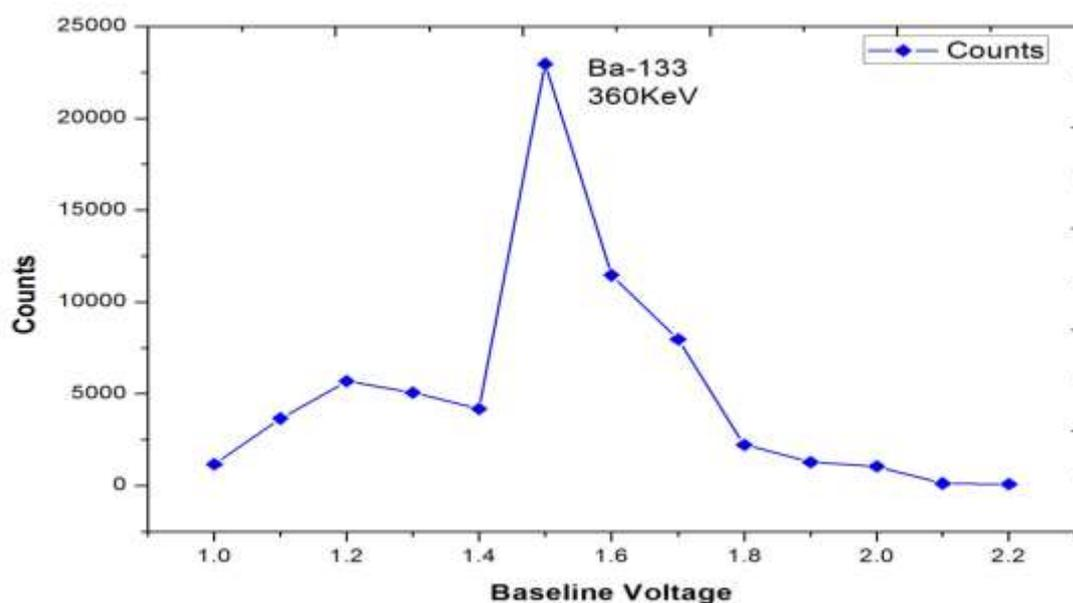
**Fig. 2. A typical spectrum of gamma-ray without attenuation for Ba-133**
