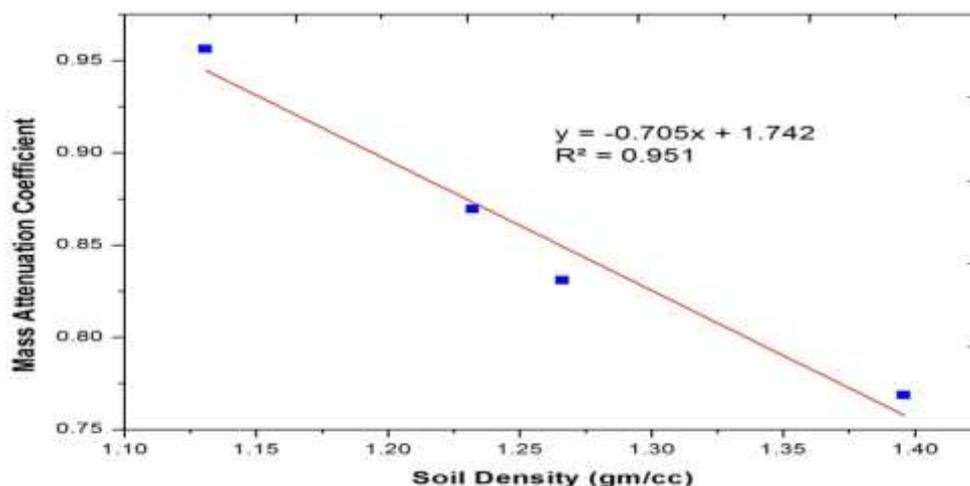
**Fig.4. Mass attenuation coefficient versus the soil density at 360 keV**
