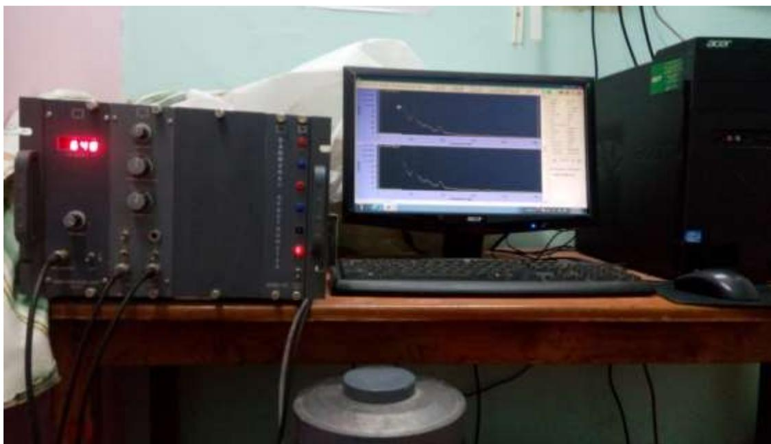
**Fig.1. Photograph of experimental set-up of attenuation of gamma-ray**
