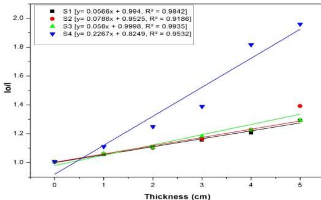
Fig.3. The thickness versus  $I_0/I$  for the investigated soil samples
