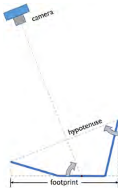
Figure 3. Schematic of a solar cooker side view, in blue, and reference lines, in gray, for determining the solar cooker elevation angle (gray arrows).
