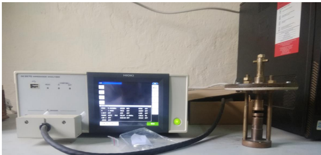
Fig- 2 LCR-Q meter (impedance analyzer model IM3570) with solid sample holder
