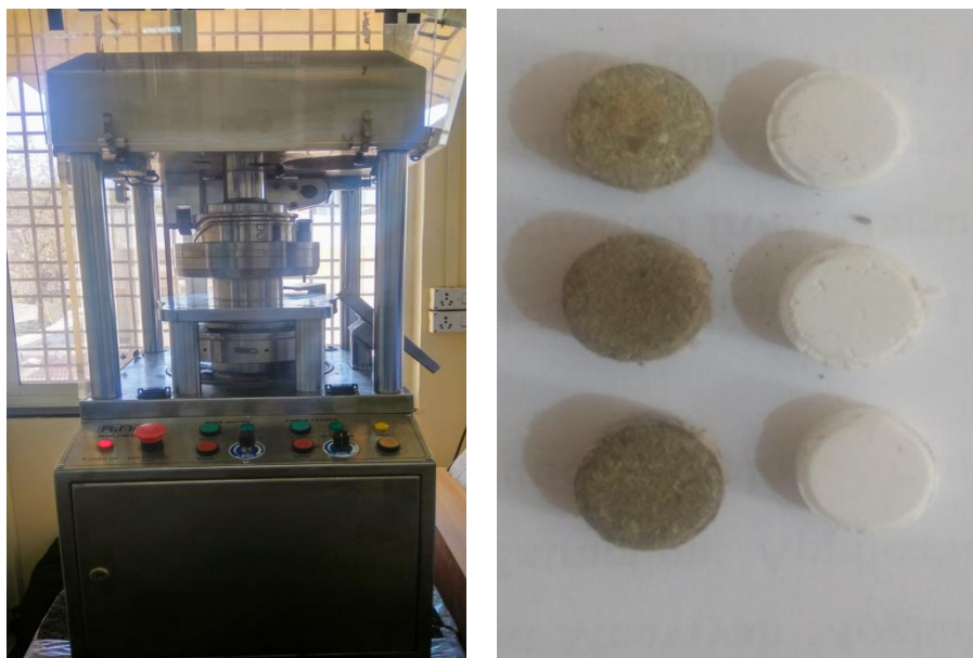
Fig- 1 shows the pallets prepared by different drug powder Standard tablet machine at constant pressure and dimension
