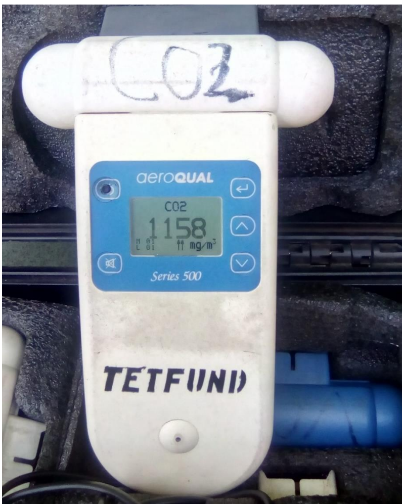
Fig 4: Aeroqual Series 500 Digital Gas Analyzers
