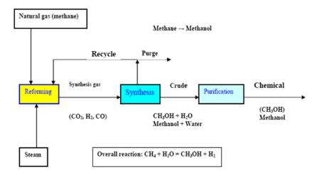
Figure 2. Schematic diagram shows methanol production (Omer, 2006).
