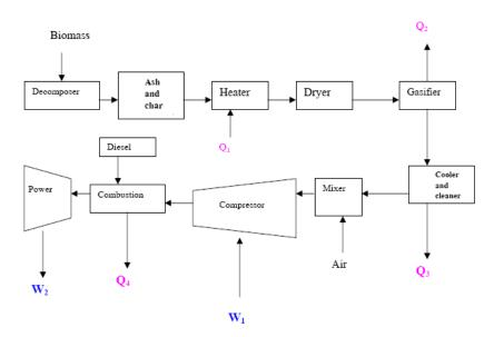
Figure 7. Advanced biomass power with diesel engine (Omer, 2006).
