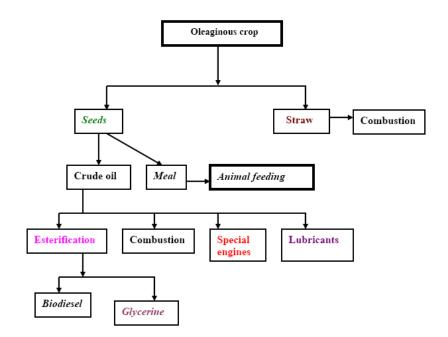
Figure 9. Flow chart of biodiesel production (Omer, 2006).
