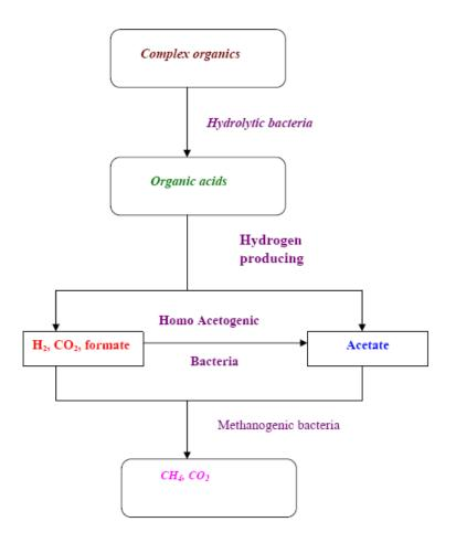
Figure 3. Biogas production process (Omer, 2003).
