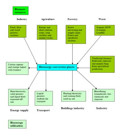
Figure 4. Biomass resources from several sources are converted into a range of products for use by transport, industry and building sectors (Sims, 2007).
