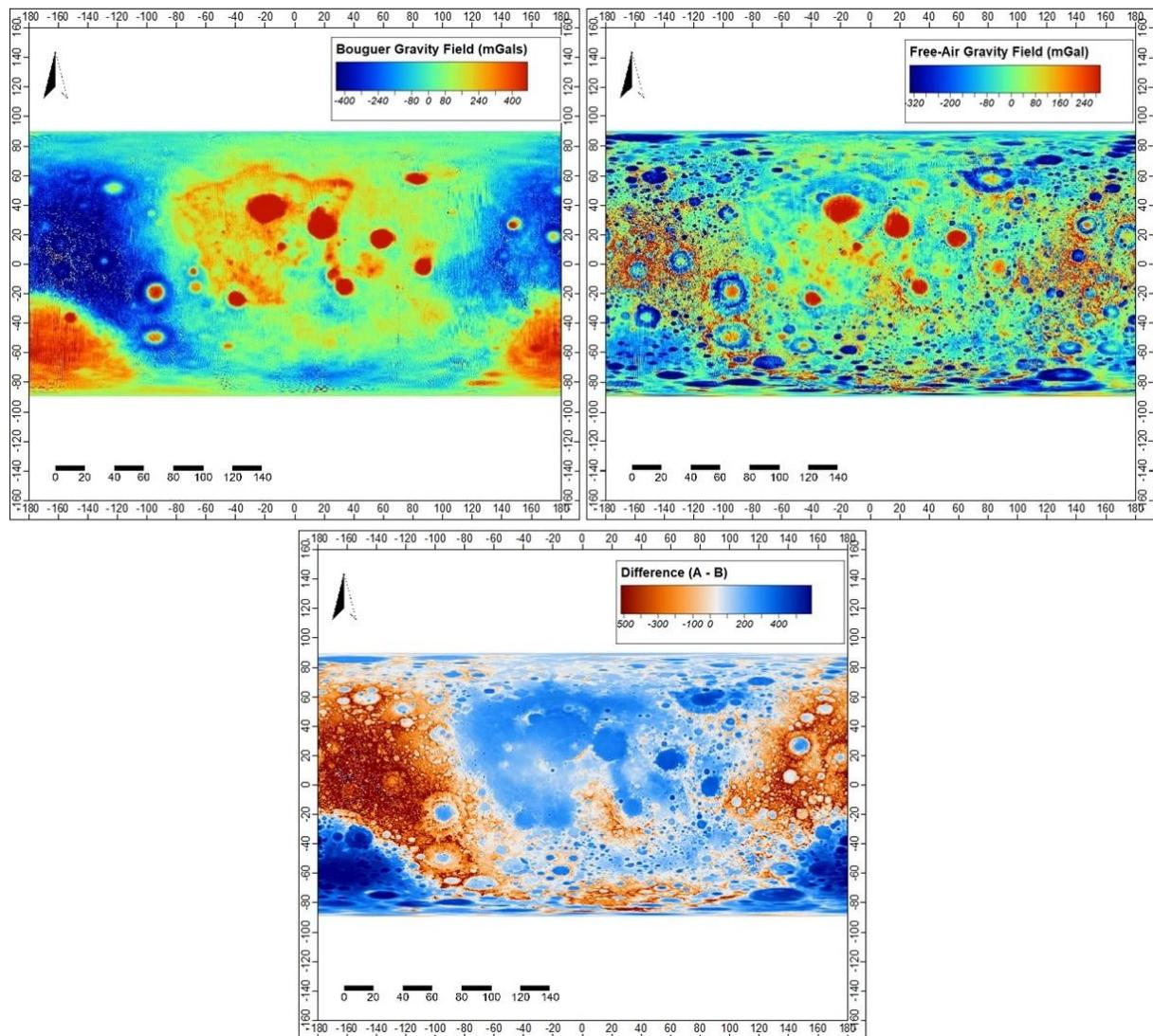
Fig.3: Comparison between lunar Free-Air and Bouguer gravity fields data using Standard Deviation (SD) approach. It is evident from the figure that there are serious differences in the absolute values of both types of gravity.
