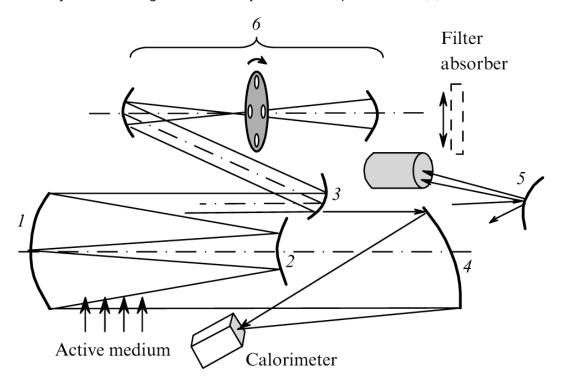
**Figure 1.** Scheme of the experimental setup: (1, 2) mirrors of the unstable resonator; (3) mirror coupler; (4) rotatory mirror; (5) deflecting mirror; (6) system for the formation of an injected beam.
