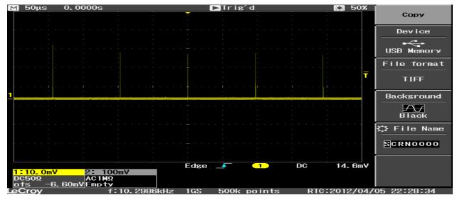
Figure 5. High repetition rate P-P mode of operation for high power Nd YAG laser.
