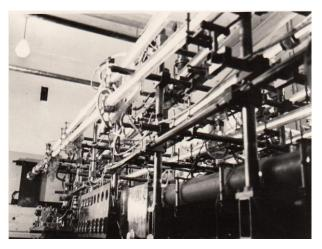
Figure 7. "Zig-Zag"- CO<sub>2</sub>-laser created by A.I. Barchukov FIAN 1970.
