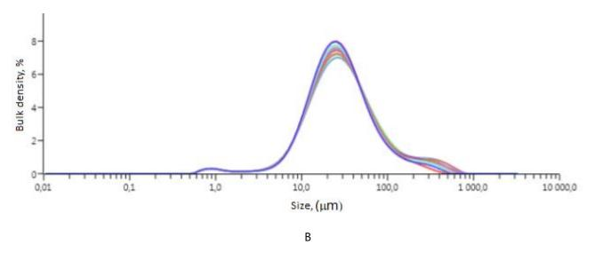
Fig. 2. The distribution of the particles for samples PFA (A) and PFB (B) determined by lazer diffraction.
