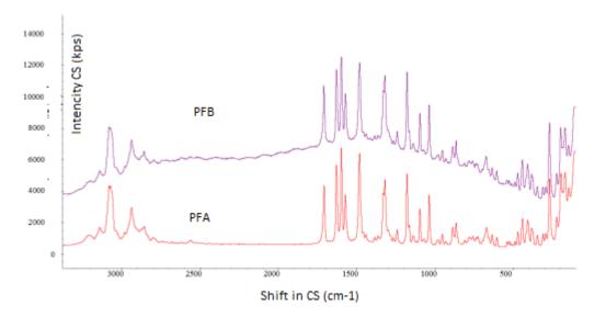
Fig. 4. Combination scattering spectra for samples PFA and PFB.
