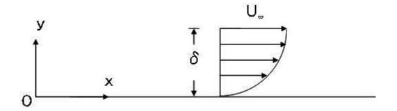
Figure 9 Definition sketch of flow past a flat plate at incident angle of zero.
