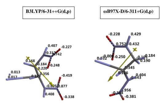
Figure 2. The ESP charges (esu) on atoms of EDNA+p system.
