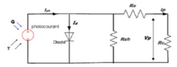
Fig 3 Equivalent circuit of a solar cell
