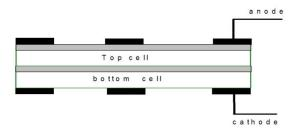
Fig. 1 Equivalent diagram of a solar cell Tandem
