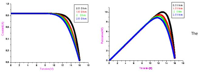
Fig.10: the influence of the series resistance on the characteristic  $I\left(V\right)$  for the panel tandem
