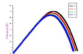
Fig.9: The influence of temperature on the characteristic P (V) for the panel Tandem
