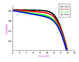
**Fig.13:** The influence of the series resistance on the characteristic
