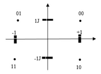
Figure.1. Constellation Diagram of QPSK
