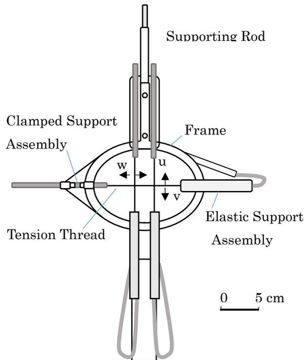
**Fig.1 Present Tension Thread Flow Meter model.**
