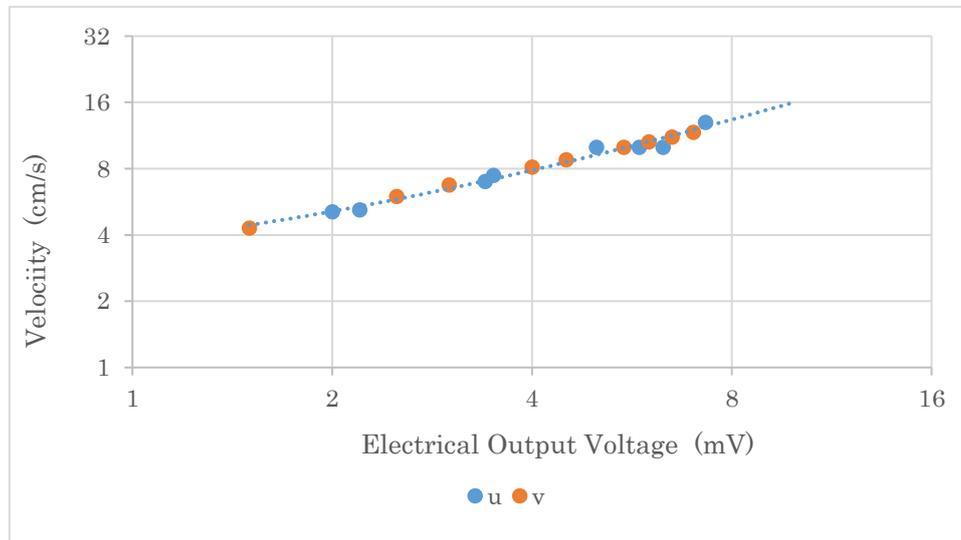
**Fig.2 Velocity calibration curve for present Tension Thread Flow Meter.**
