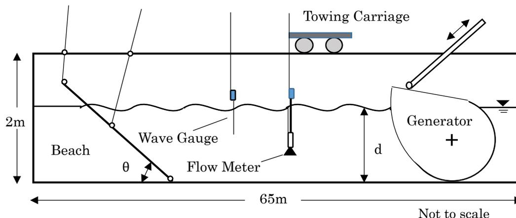
**Fig.3 Schematic diagram for the present experiment.**
