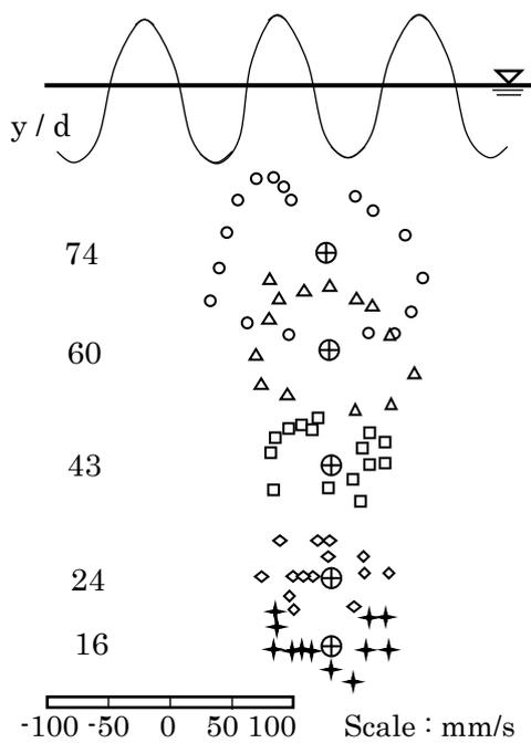
**Fig.5 Time histories of the water particle velocity vector for wave 2 at each normalized vertical distances.**
