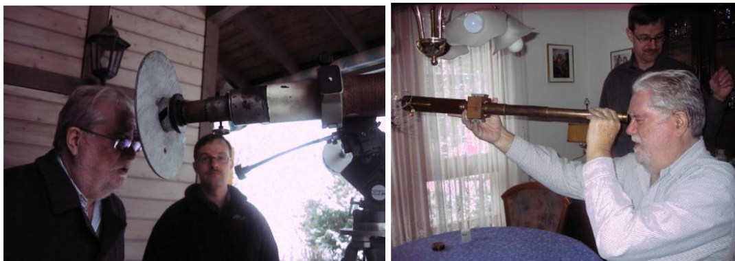
Figure 40. (Left) The 82 mm aperture (magnification X64) refractor used mostly by Wolf's assistants at the Zürich Observatory since 1864, designed by Joseph Fraunhofer and manufactured in 1822 at the Fraunhofer factory by his assistant Georg Merz. The telescope still exists and is being used daily by Thomas Friedli (person at center). (Right) One of several small, portable, handheld telescopes (~40 mm aperture, magnification X20) used by Wolf almost exclusively from 1860 on, and still in occasional use today. More on the telescopes can be found at Friedli [2016]. (Photos: ).
