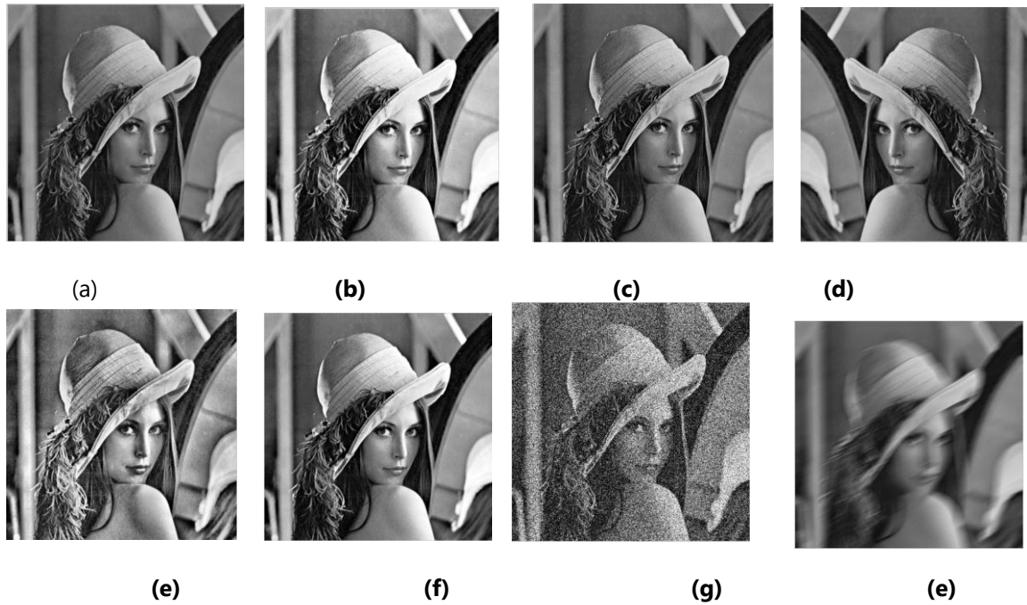
Fig. 8: Watermarked image 'Lena' with different attacks (a) Original image. (b) Histogram equalization attack. (c) Sharpening attack (d) Flipping attack (e) Blurring attack (f) Contrast adjustment attack (g) Gamma correction attack (h) AWGN attack.
