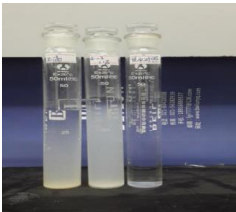
FIG. 5. Effect of sample suspension by different titration methods after sedimentation for 24 h. the samples
