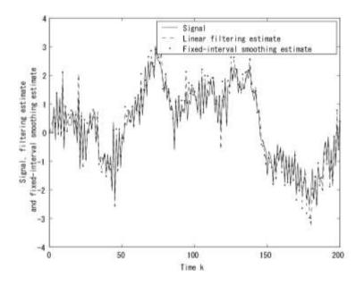
Fig.2 Signal, robust RLS Wiener filtering estimate by Nakamori [10] and fixed-interval smoothing estimate by Nakamori et al. [12] for white Gaussian observation noise  $N(0, 0.3^2)$ .
