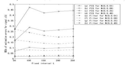
Fig.3 MSVs of filtering and fixed-interval smoothing errors by robust RLS Wiener filter [10] and RTS fixed-interval smoother [13], [14] vs. fixed interval L.
