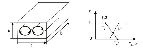
Figure 1 Thermal convection in a box at flow regime of thermally strained quiescence.
