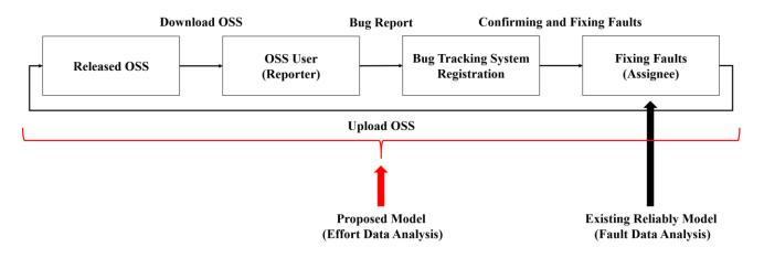
Figure 1: The OSS development using bug tracking system.
