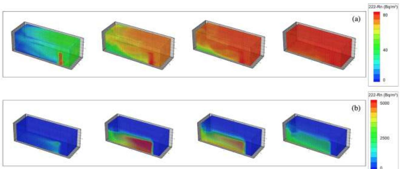
Fig. 4. Tecplot 360 [16] rendering of radon concentration in the living room simulated with CFD-0 considering (a) steady weather conditions and (b) variable weather conditions including wind. The same 2h period as in Fig. 3 was used.
