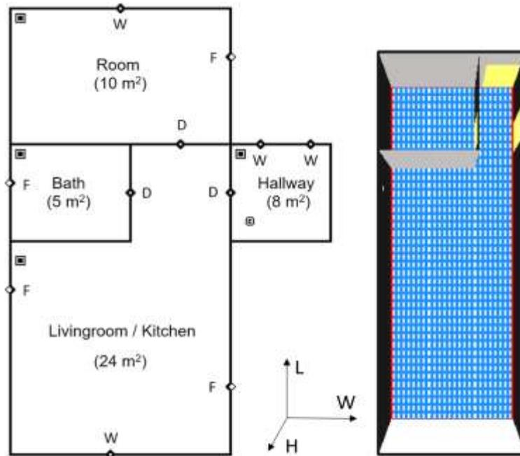
**Fig. 1.** (a) CONTAM and (b) CFD-0 drawings of the entire dwelling and bath together with the living room.
