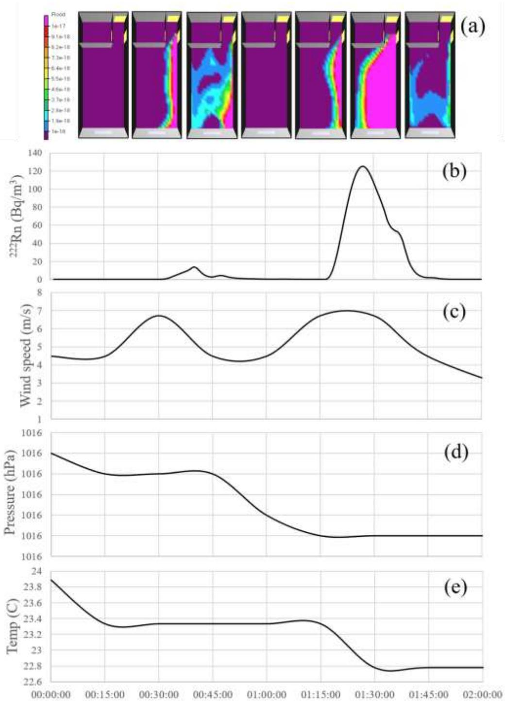
**Fig. 3.** Radon concentration in the living room simulated with (a) CFD-0 and (b) CONTAM for a 2h period. The outdoor conditions which have been shown to have a significant impact in the radon concentration are displayed, such as (c) wind speed, (d) pressure and (e) temperature.
