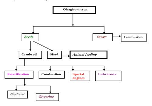
Figure 9. Flow chart of biodiesel production (Omer, 2006).
