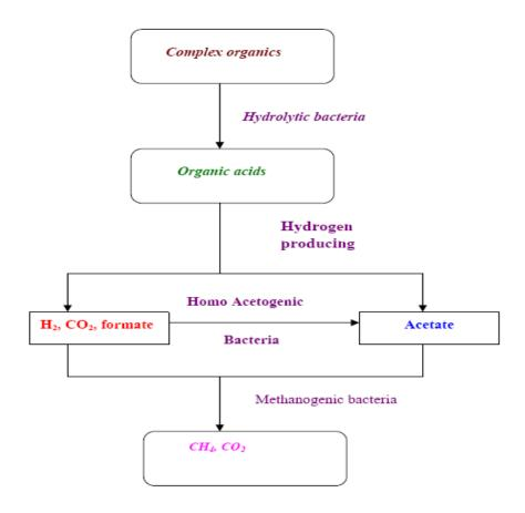
Figure 3. Biogas production process (Omer, 2003).
