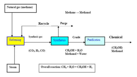
Figure 2. Schematic diagram shows methanol production (Omer, 2006).
