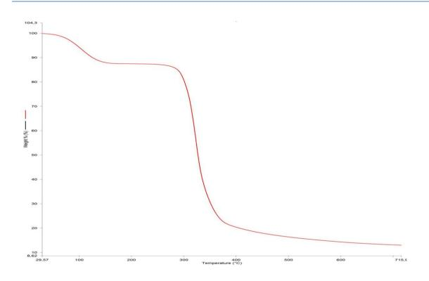
Figure 4(a): Thermo-gravimetric Analysis (TGA) Spectrum of Modified Poly (ester amide)
