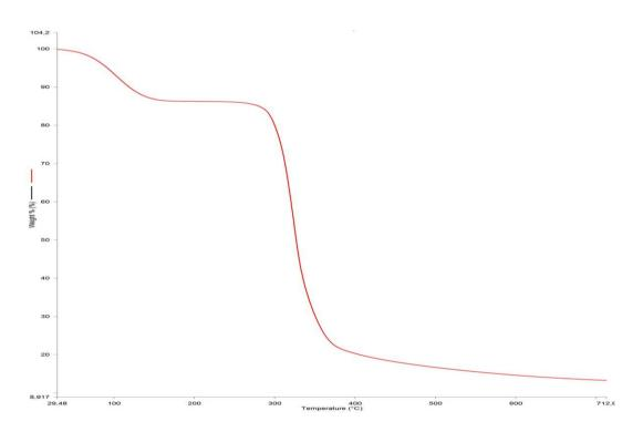
Figure 3(a): Thermo-gravimetric Analysis (TGA) Spectrum of Unmodified Poly (ester amide)
