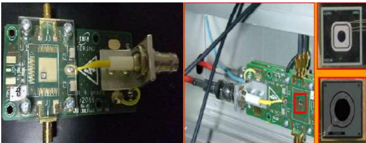
Figure (2): A pair of sensor board, Ultra-Fast Silicon Detectors ( $1 \text{ mm}^2 \times 50 \mu\text{m}$ ).
